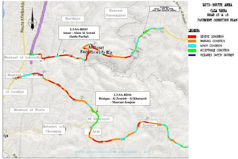
Figure 3-5: Pavement Condition Plan of Road L3-SA-RD15 and Road L3-SA-RD16 in Saida Caza
