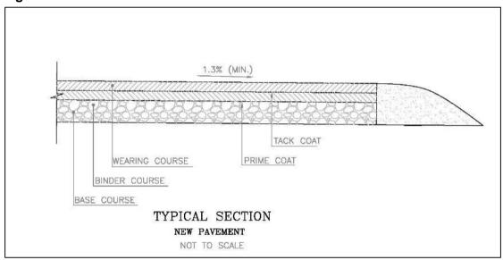
Figure 3-11: New Pavement Cross Section Scheme
