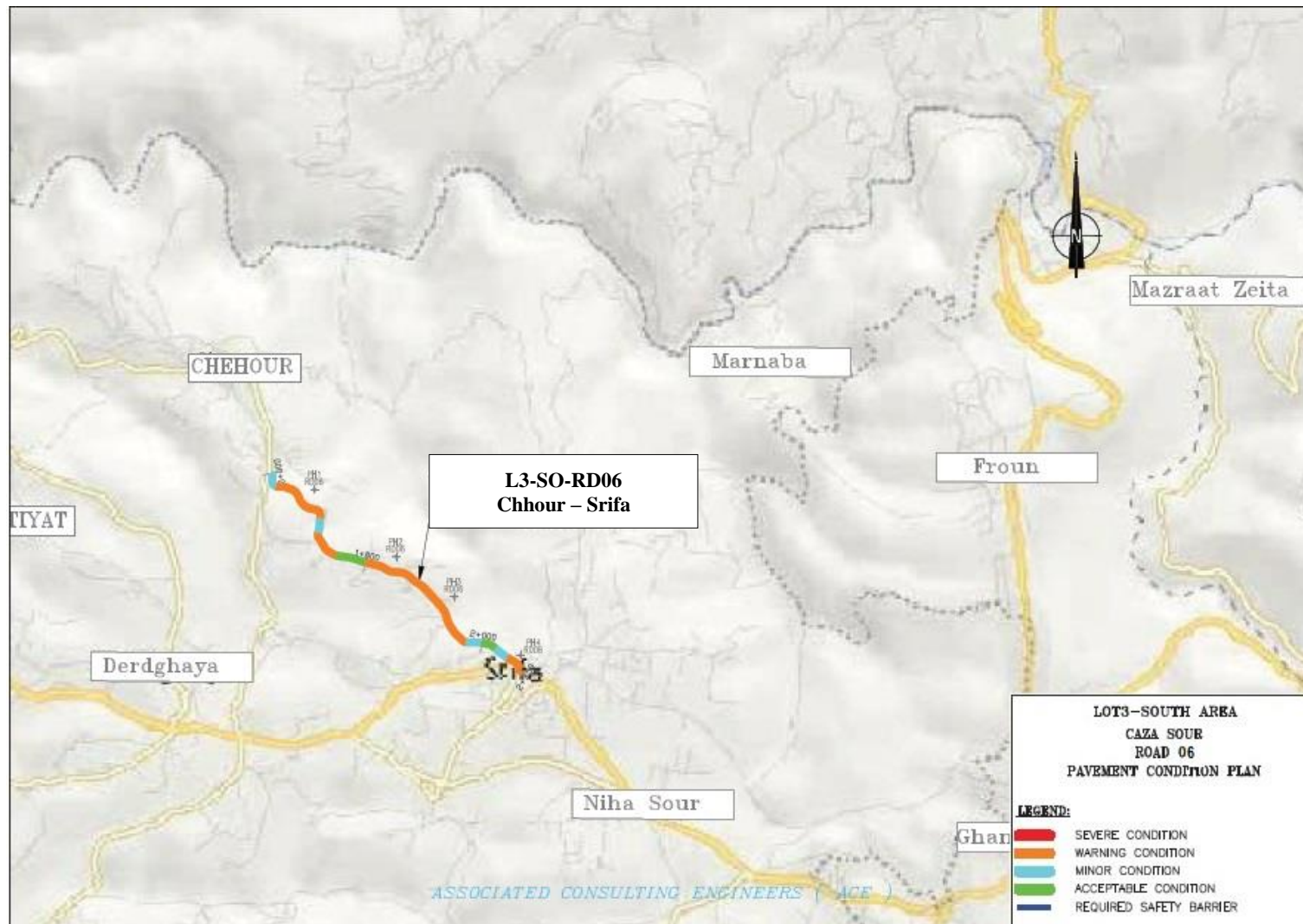
Figure 3-5: Pavement Condition Plan of Road L3-SO-RD06 in Sour Caza
