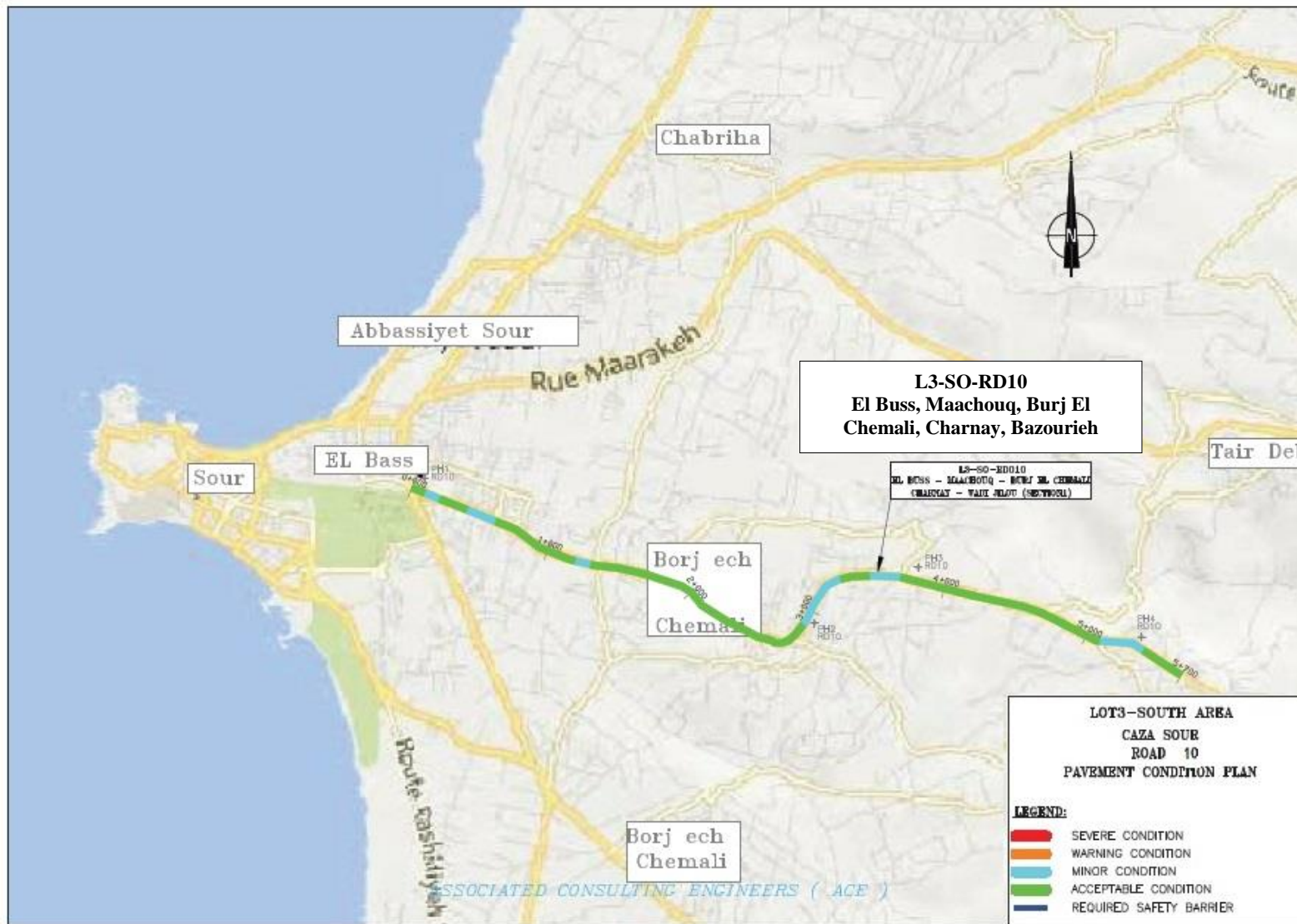
Figure 3-11: Pavement Condition Plan of Road L3-SO-RD10 in Sour Caza
