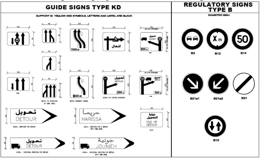
Annex 3: Road Signs, Markings, Lights, and Barricades to be Used during Rehabilitation Works
