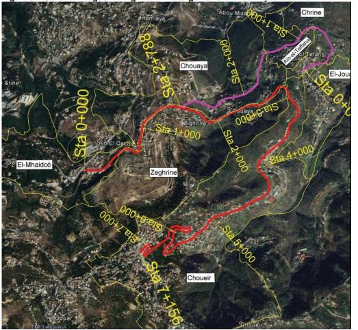
Figure 3-2 Satellite image showing Metn R1a alignments with surveyed stations
