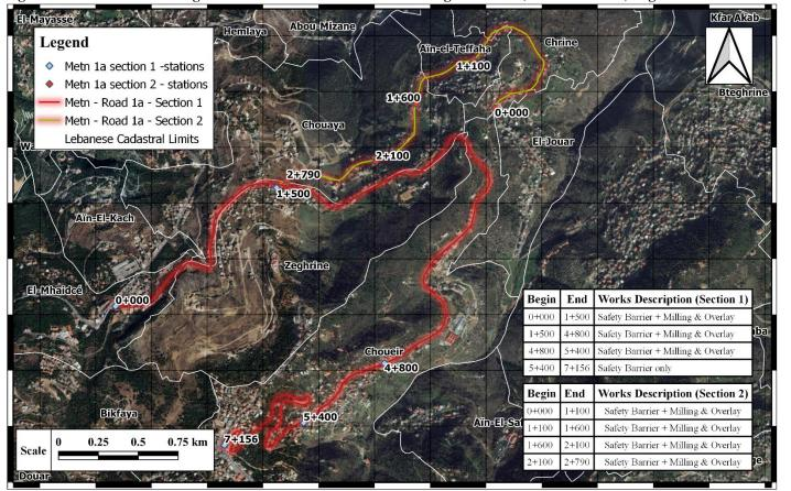
Figure 3-6 Work stations along with road rehabilitation activities along Metn R1a (sections 1 and 2) alignment
