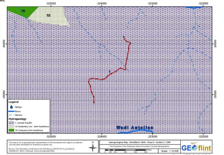
Figure Q Hydrogeological map of Metn R3 section 2 and its surrounding (map showing water potential of the subsurface). Refer to Table 4 8 for description of hydrogeology classes.
