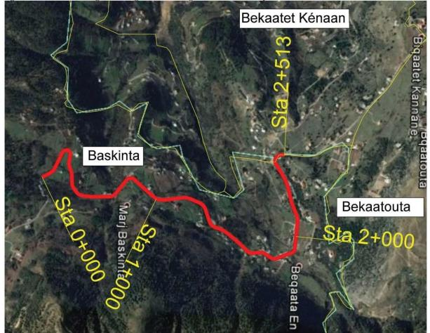
Figure 3-5 Satellite image showing Metn R4 alignment with surveyed stations
