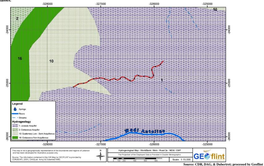
Figure O Hydrogeological map of Metn R2 a and its surrounding (map showing water potential of the subsurface). Refer to Table 4 8 for description of hydrogeology classes.
