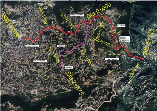
Figure 3-4 Satellite image showing Metn R3 alignment with surveyed stations
