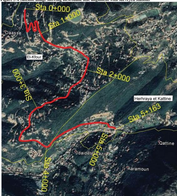
Figure 3-4 Satellite image showing Kesrouane R2c alignment with surveyed stations
