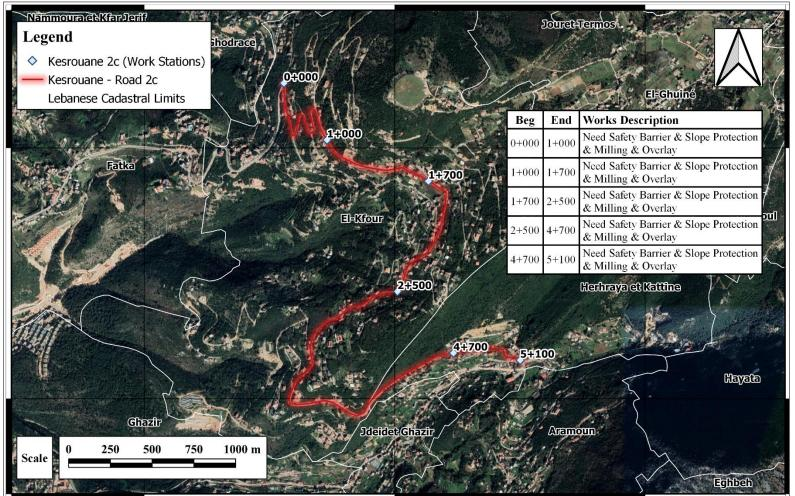
Figure 3-8 Work stations along with road rehabilitation activities along Kesrouane R2c alignment
