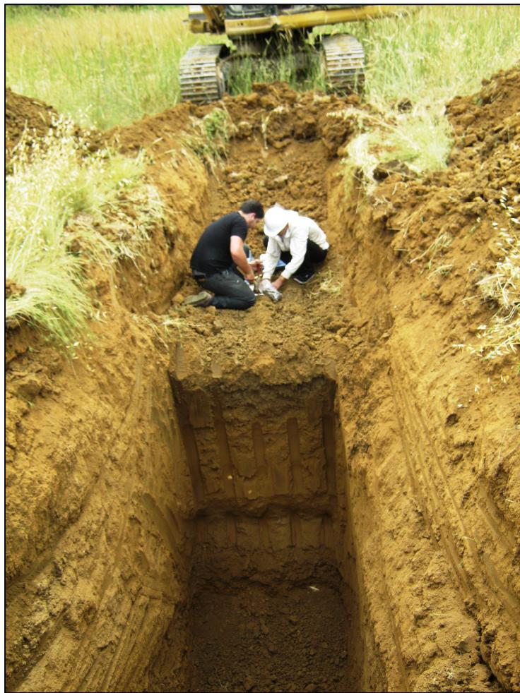
Figure 8: NTP8 (stepped pit), clay-core material source of S1-A/B/C
