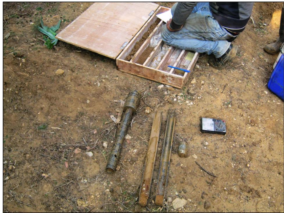
Figure 21: SPT sampler
