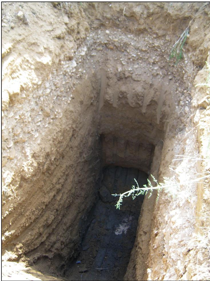
Figure 6: NTP6, clay-core material source of N-3
