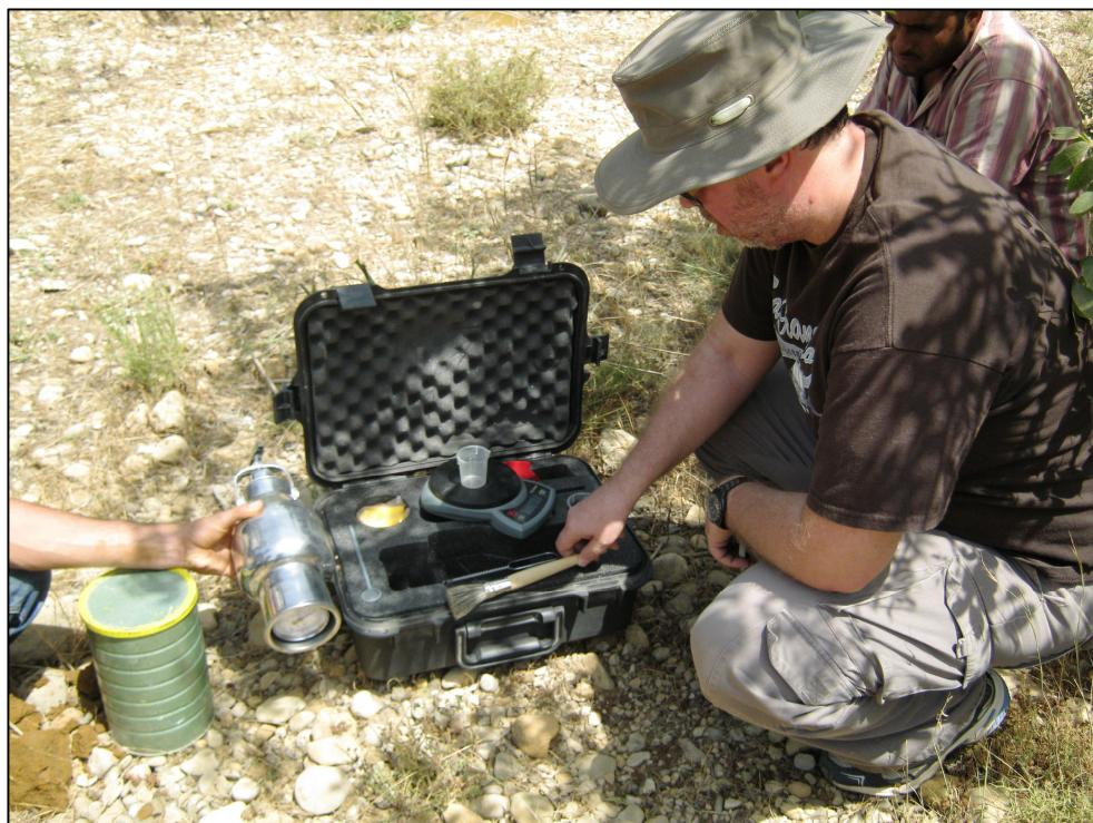
Figure 14: Speedy moisture test kit (NTP2).
