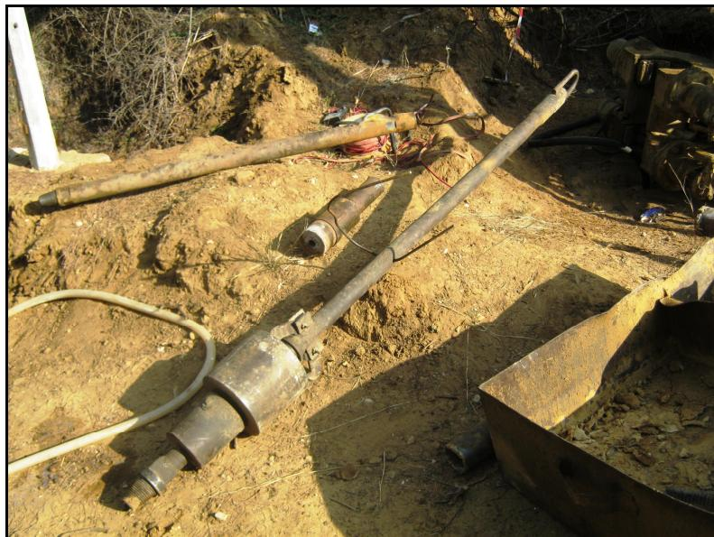
Figure 22: Automatic trip SPT hammer.
