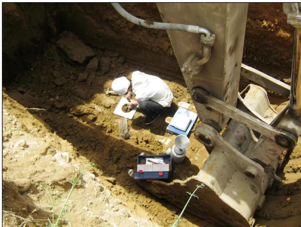
Figure 13: Sand-cone method (NTP4)
