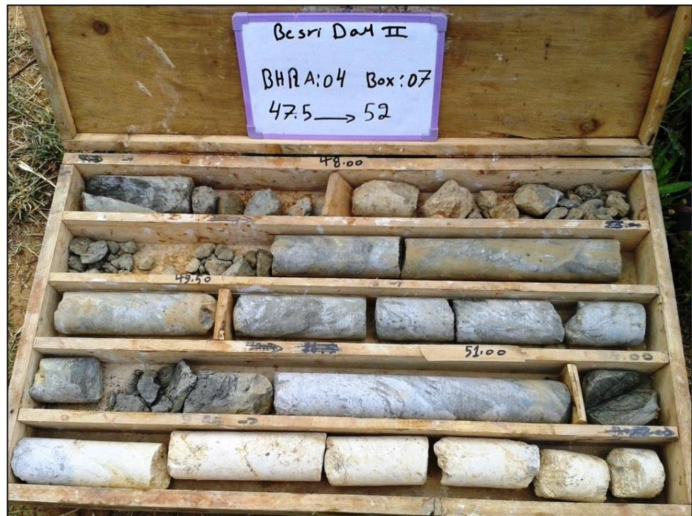
Figure 20: Standard wooden core boxes
