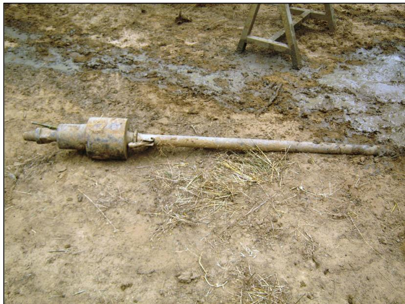
Figure 8: Automatic trip SPT hammer.
