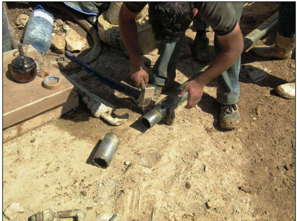
Figure 4: Double tube core barrel
