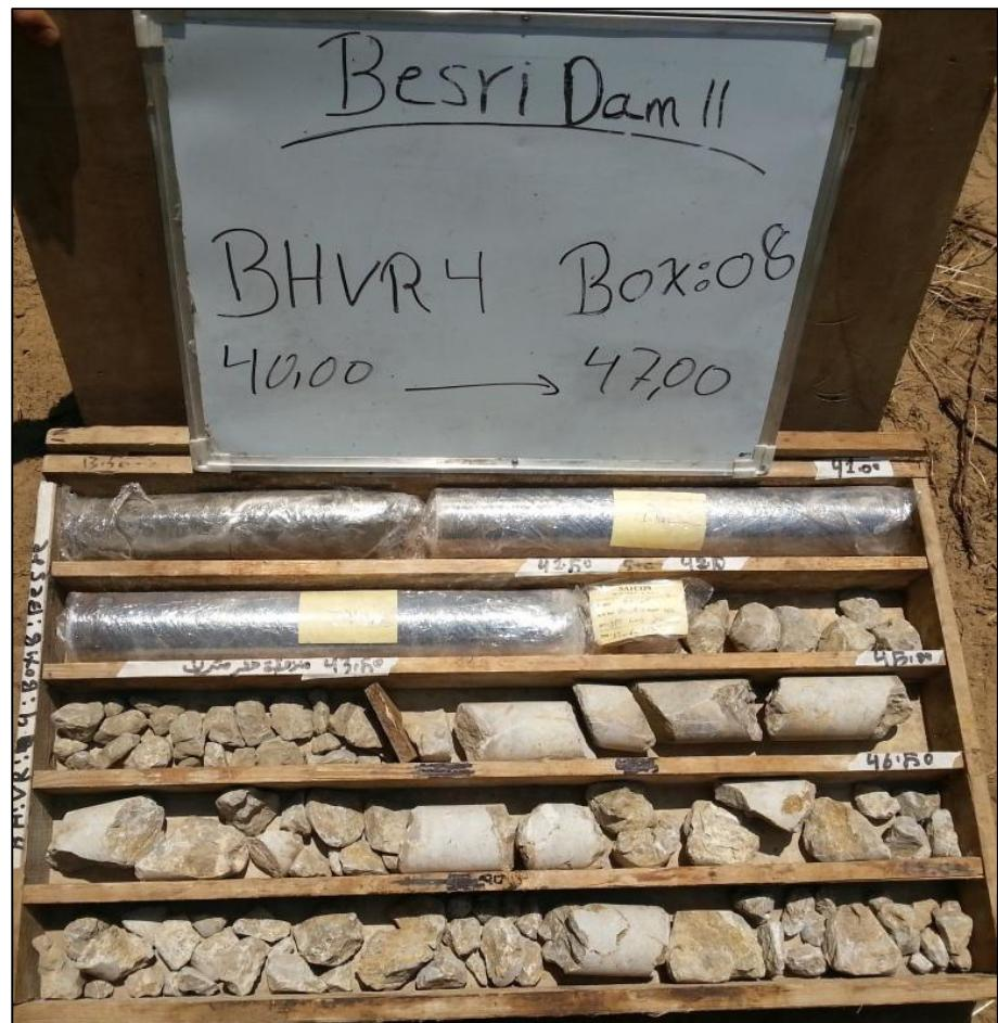
Figure 6: Standard wooden core boxes
