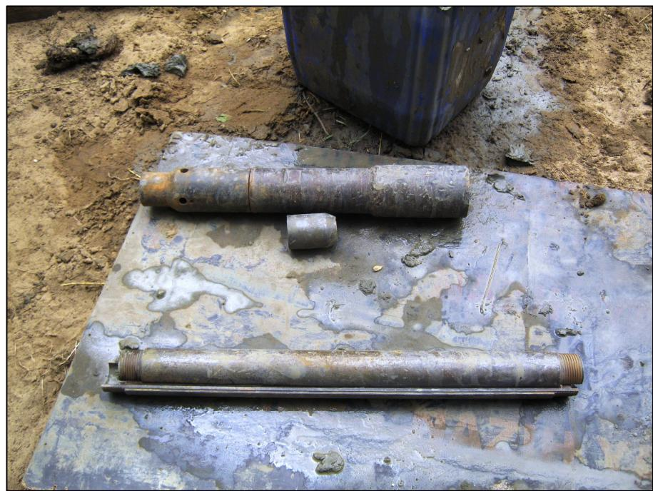
Figure 7: SPT sampler
