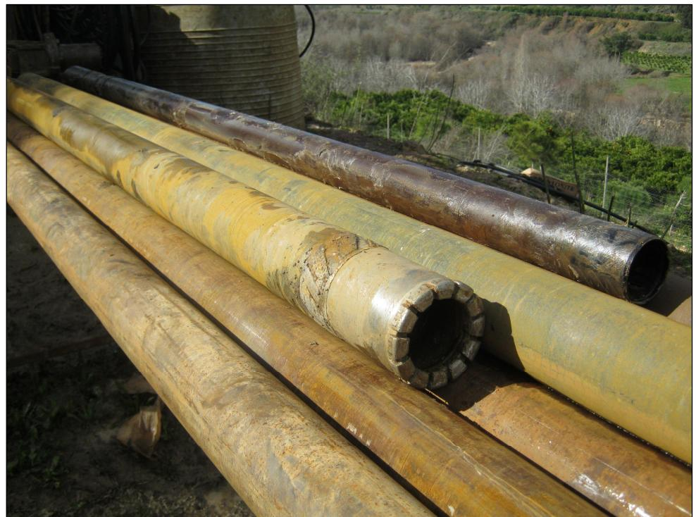
Figure 5: Wireline core barrel
