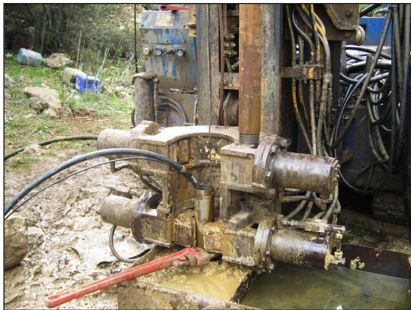
Figure 9: Multistage Lugeon Test
