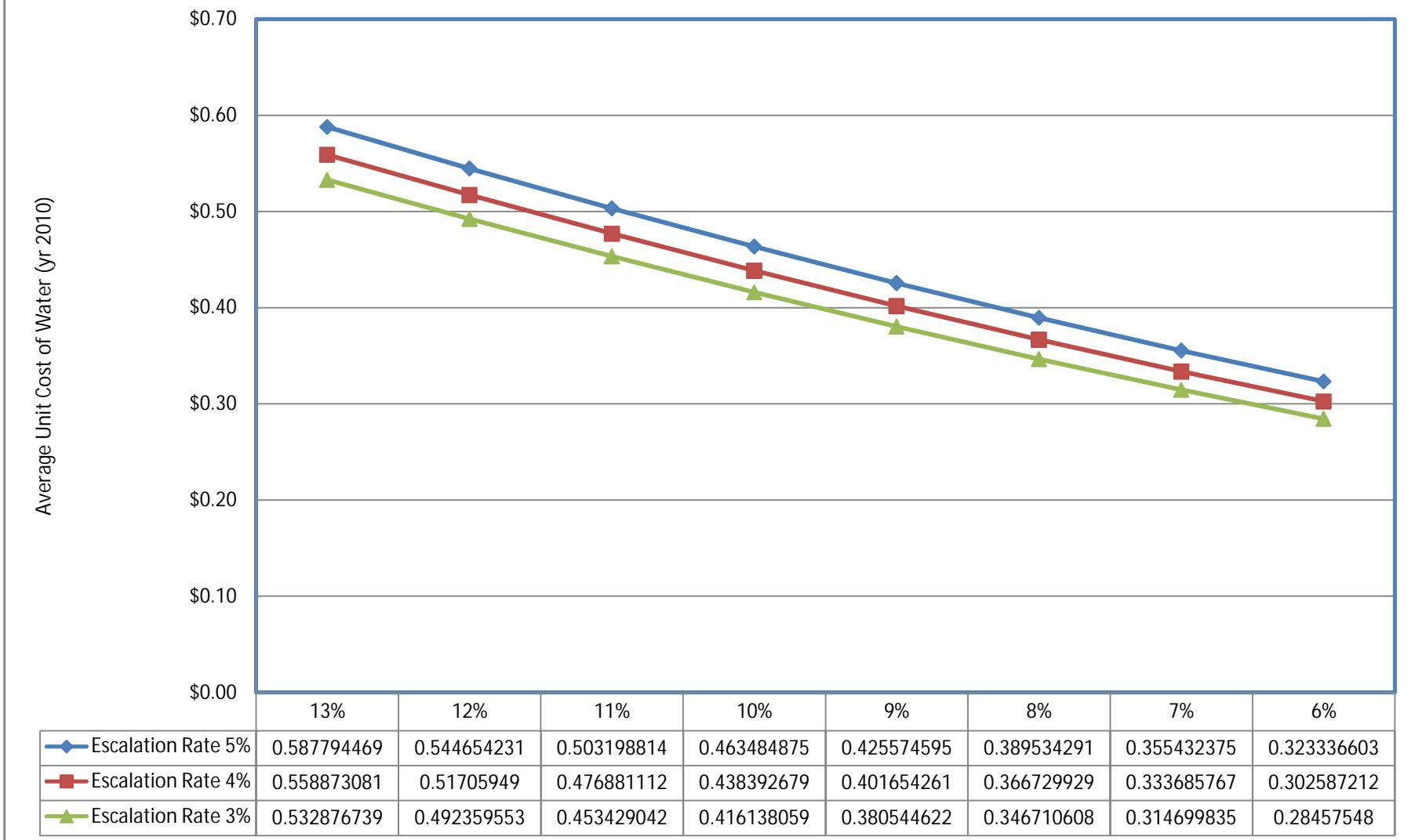
Figure 6.17: Average Unit Cost of Water (Actual)
