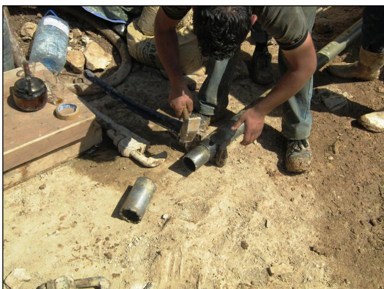
Figure 29: Double tube core barrel
