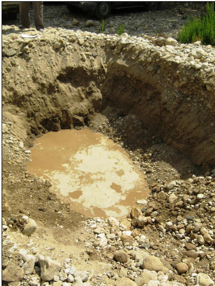
Figure 14: NTP22, Sand/Gravel material source of R-5
