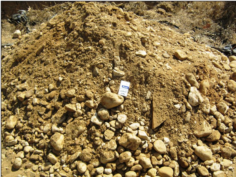
Figure 16: SAND and GRAVEL with some Cobbles (NTP11).
