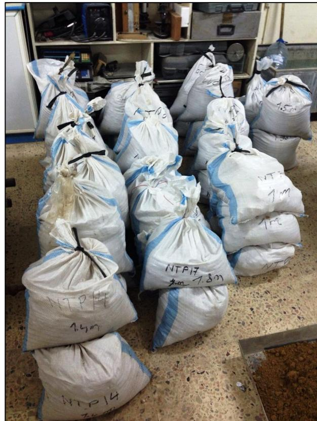
Figure 26: Bulk samples taken from the new test pits (NTP9-NTP23).
