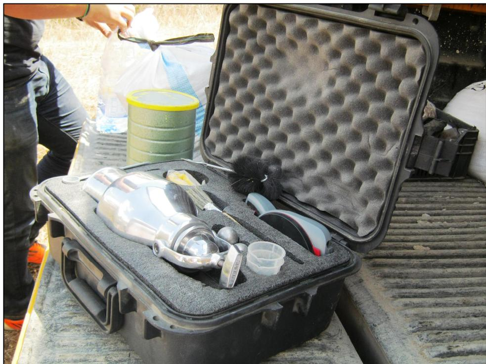
Figure 24: Speedy moisture test kit.
