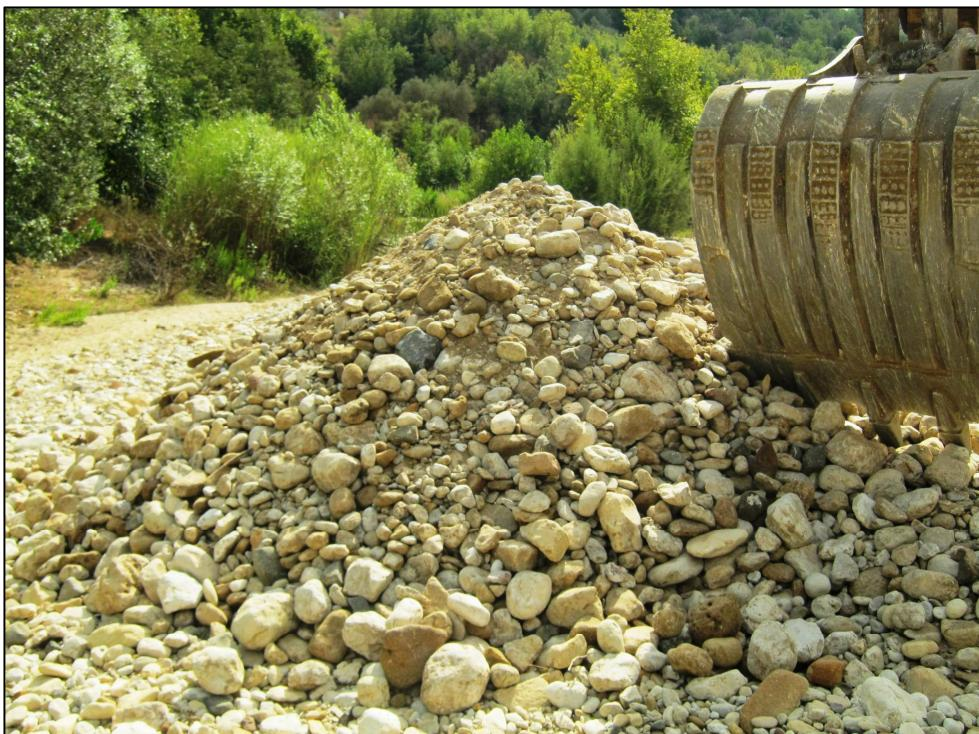
Figure 17: SAND and GRAVEL with Cobbles and Boulders (NTP23)
