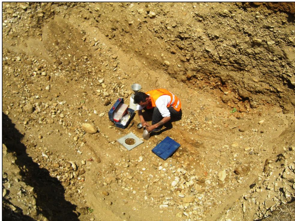
Figure 23: Sand-cone method (NTP21)
