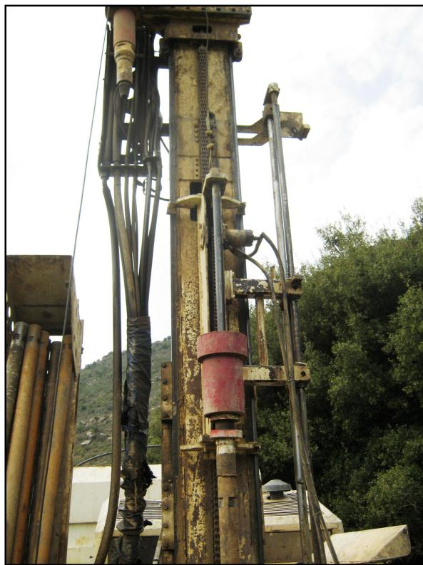
Figure 31: Automatic trip SPT hammer.
