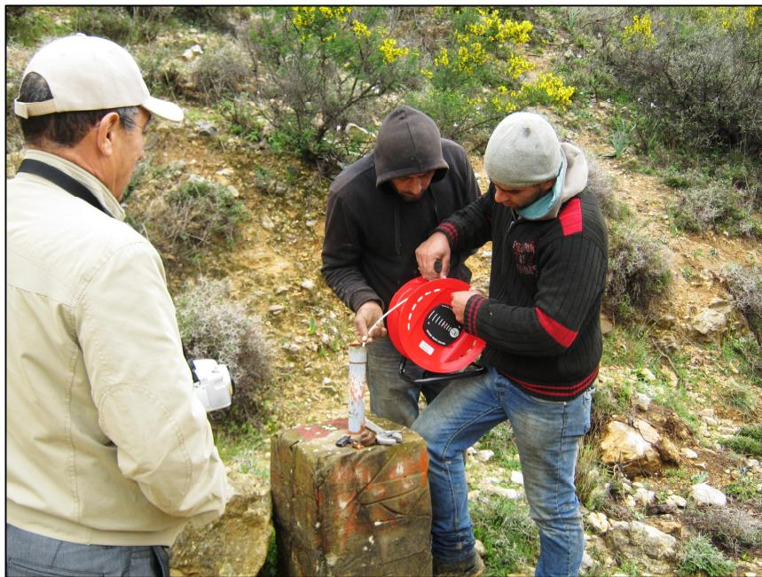
Figure 16: Measuring the depth of groundwater
