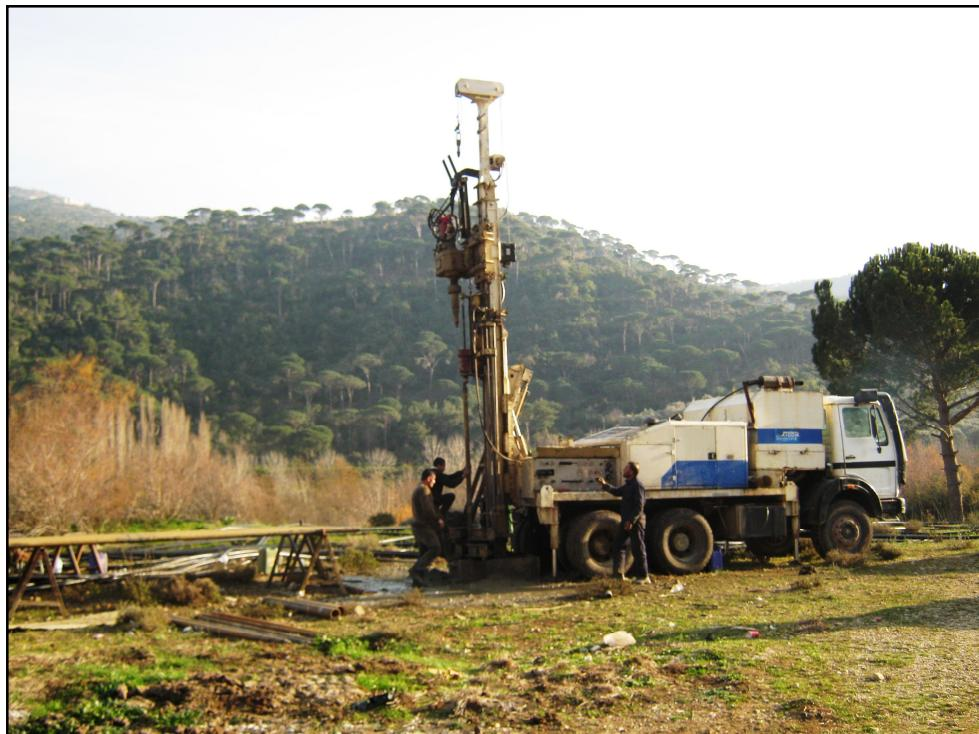
Figure 4: Truck mounted drill rig used in DCPT probing (DCPVR9).
