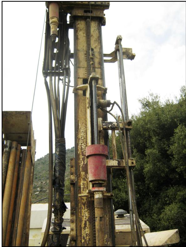
Figure 11: Automatic trip SPT hammer used in DCPT probing.
