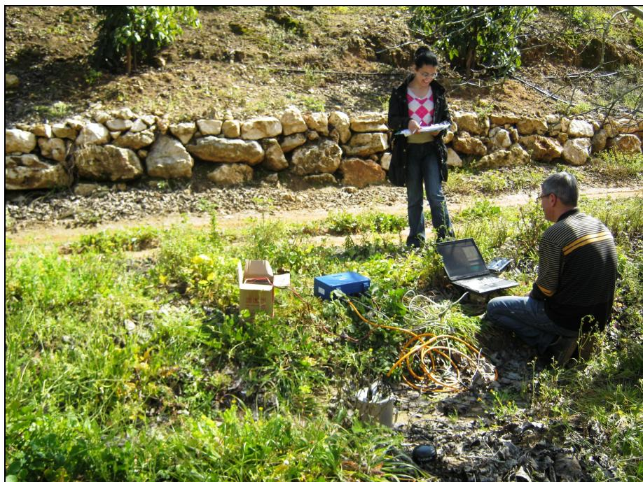
Figure 1: Ambient earth noise survey
