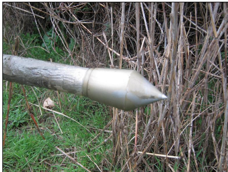
Figure 9: Solid cone used in DCPT
