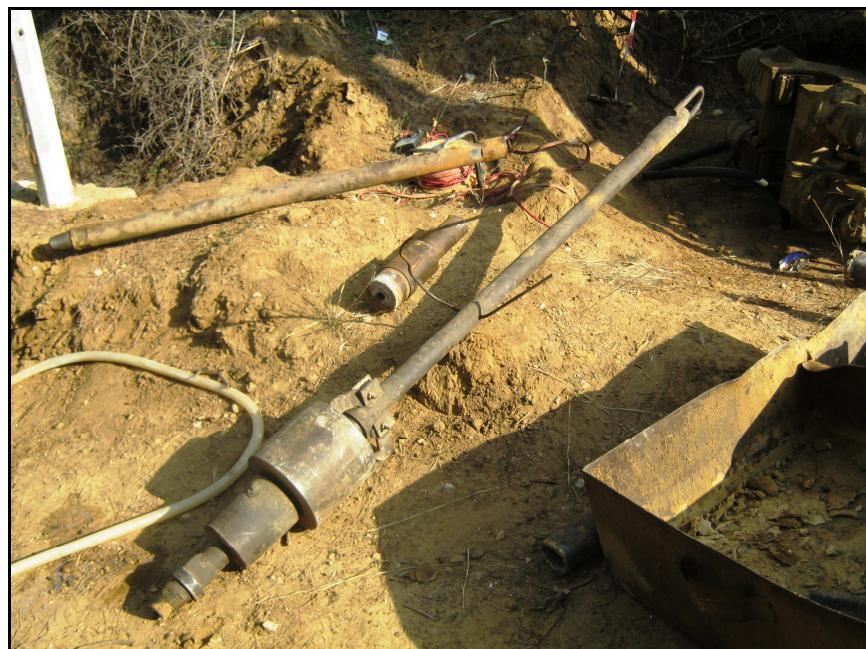
Figure 10: Automatic trip SPT hammer used in boreholes.
