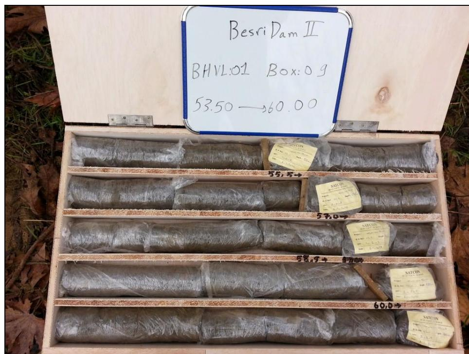
Figure 7: Standard wooden core boxes
