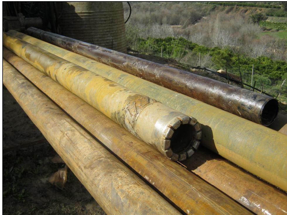
Figure 6: Wireline core barrel
