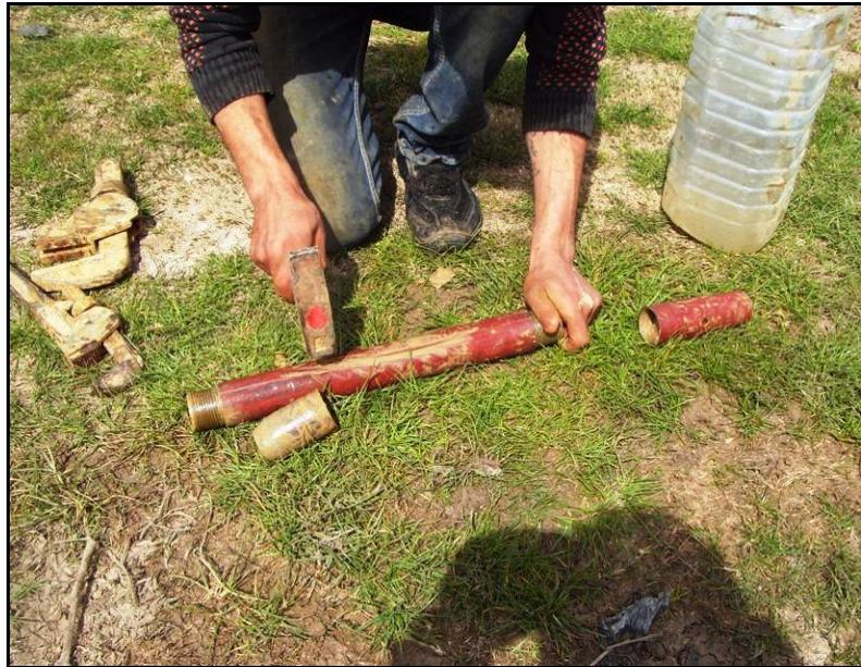
Figure 8: SPT sampler
