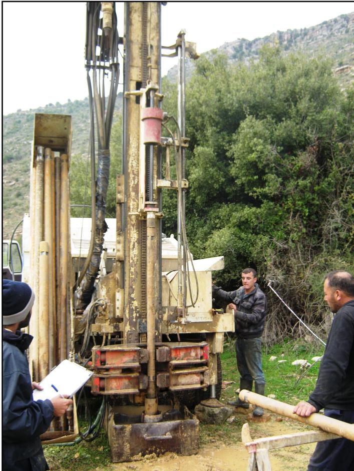
Figure 12: Continuous DCPT probing.
