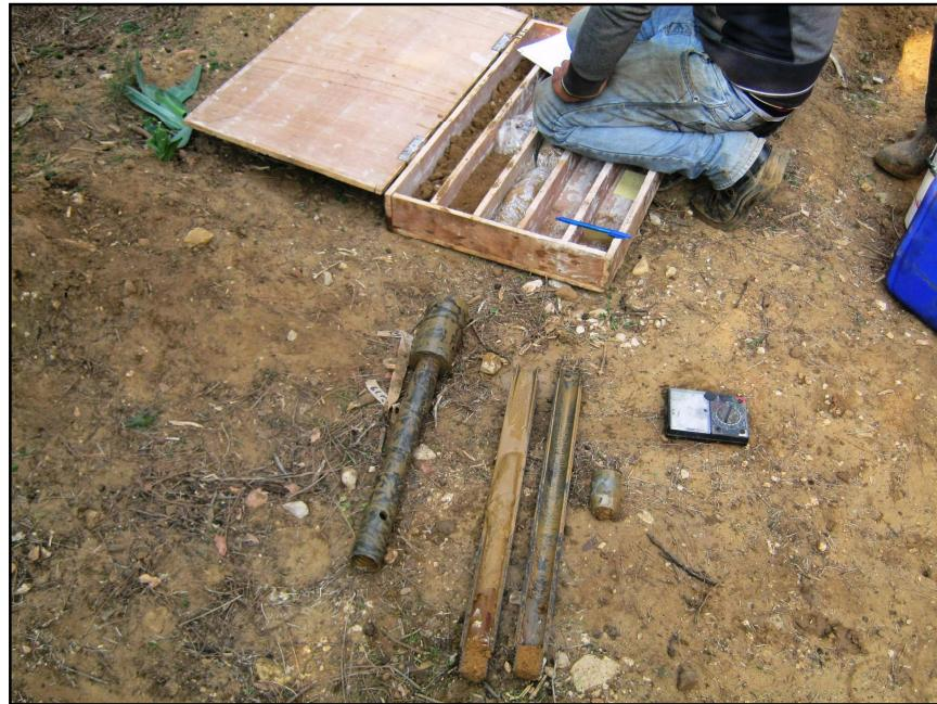
Figure 3: Wooden core box and SPT sampler
