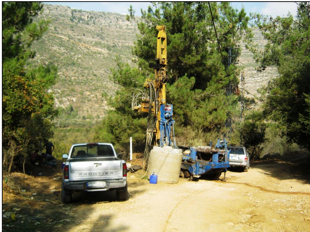
Figure 2: Crawler mounted rotary drill rig (EV1)
